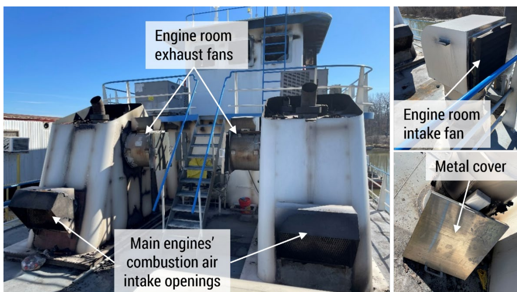
Figure 10. Clockwise from left: Johnny M exhaust stacks showing covered engine room exhaust fans and engine air intake openings (two openings under each hood); engine room intake fan (there were two intake fans—one port and one starboard); and metal cover, all located on upper deck.
