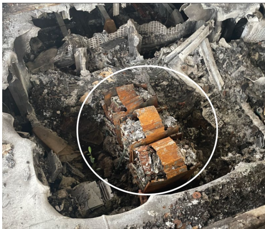
Figure 6. The 24-volt lithium-ion battery bank (circled), after the fire.
