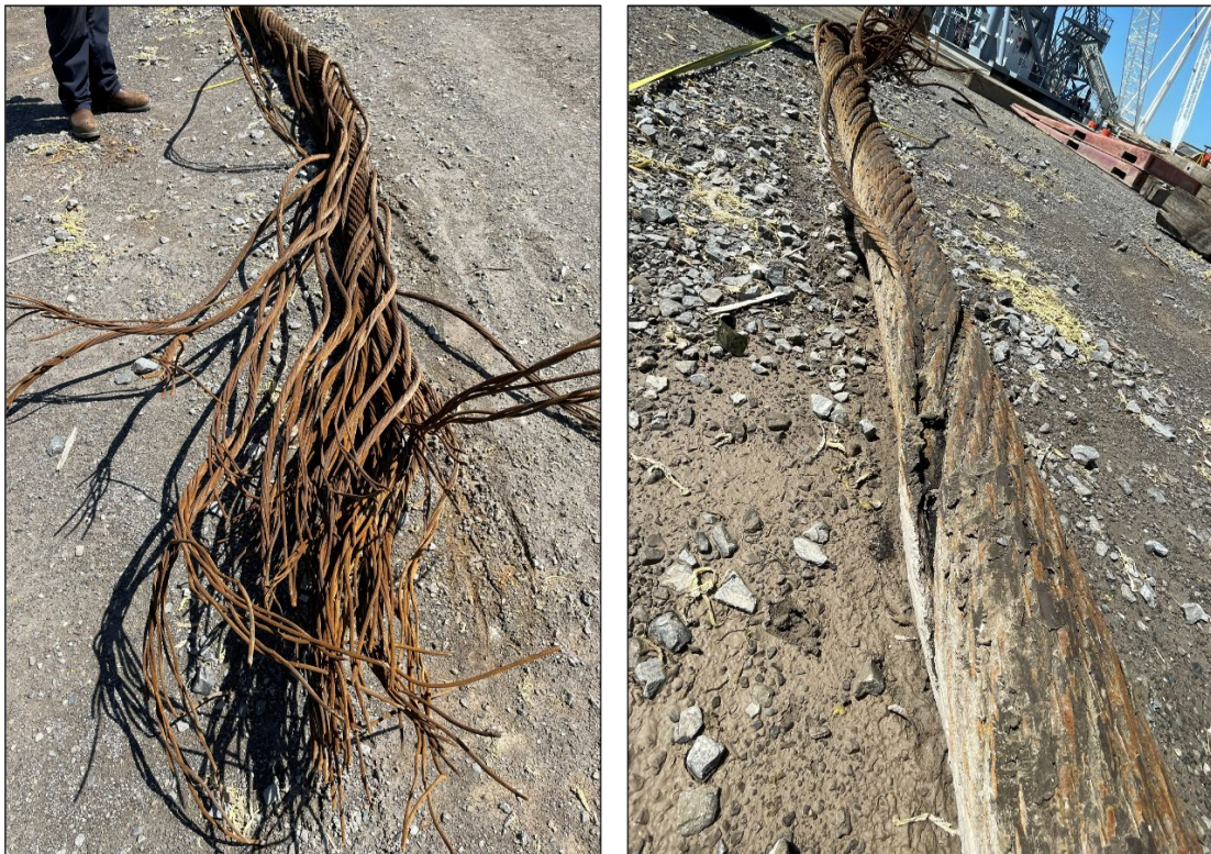
Figure 6. Parted hoisting wire that fell with wire reel onto deck of C-Enforcer .
