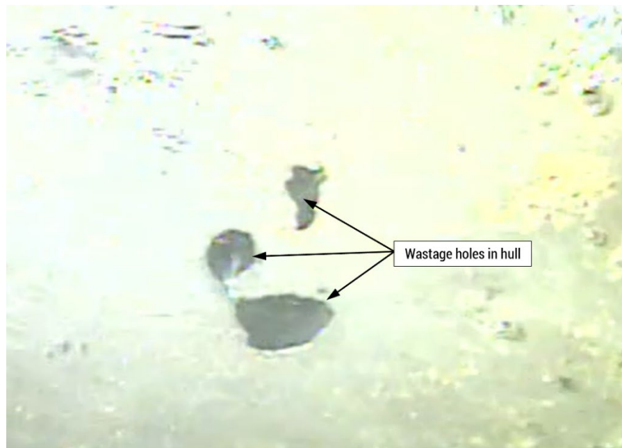
Figure 5. Wastage holes discovered in hull during postcasualty survey. (Background source: Global Diving)
